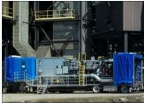
A demonstration unit built on a 48' semi-trailer that can be transported virtually anywhere in the U.S. or Canada gives potential customers an on-site demonstration of the dry Pahlman Process technology (Photo: EnviroScrub)
